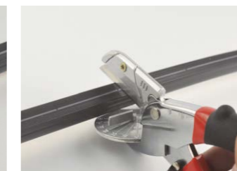
Use professional scissors to cut vertically at the cutting mark
